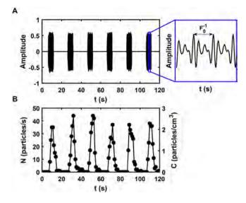
**Figure 1.** Representative raw data in which a participant (F4) said /a/ for 5 seconds, followed by 15 seconds of nose breathing, repeated 6 times at approximately the same loudness. (**A**) The amplitude (arb. units) recorded by the microphone versus time. Magnification shows 13 ms of the waveform with fundamental frequency of  $F_0$ . (**B**) The corresponding number/concentration of particles measured by the APS versus time.
