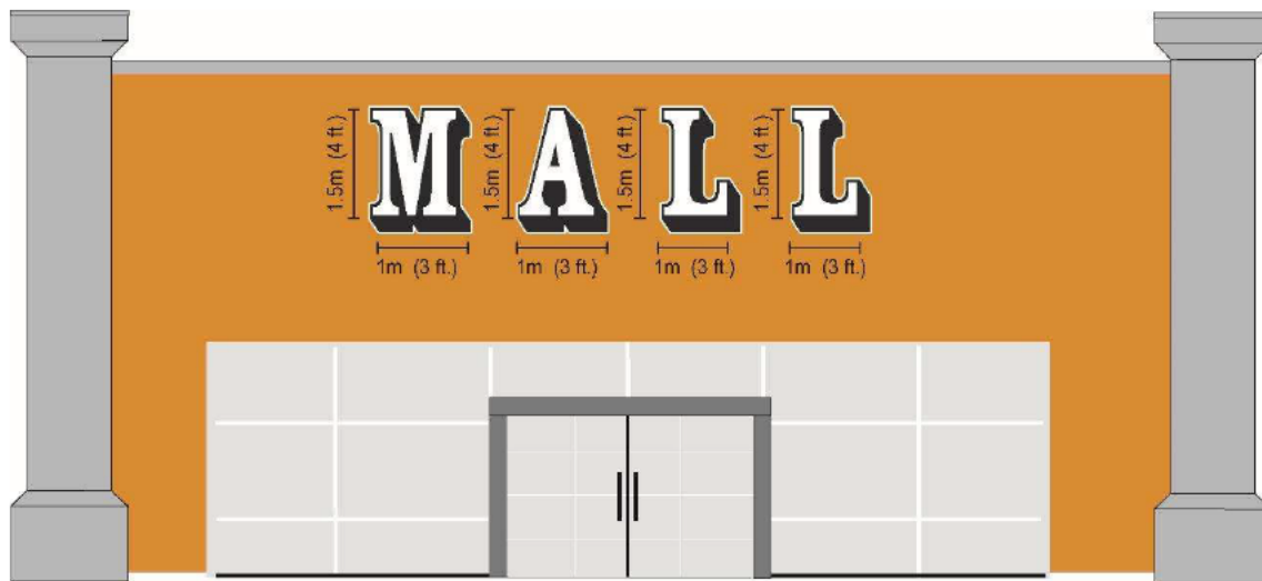
Figure 5.6.1: Determining Area of Box Sign
